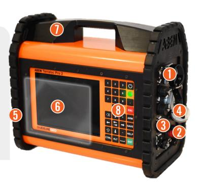
ABEM Terraloc Pro 2 is a standalone system and comes with built-in computer, data storage, measurement channels and user interface. Measurements are conducted via a user friendly graphical interface. The system is enclosed in a rugged and robust aluminum casing meeting IEC IP66 classifications, allowing measurements to be made in all situations and environments.
