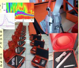
used as inclinometers and at the same time as accelerometers for dynamic motion recording.
