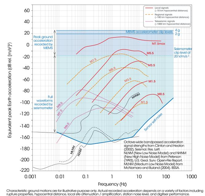
Self-noise level based on equivalent sensor from a Güralp Breve ocean bottom seismometer.
